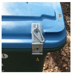
3. Lay the hinge over the lid to mark the best position for the eye of the hasp. Make sure the hinge can be locked and unlocked easily. Pre-drill  $\frac{3}{16}$  holes in the marked spots on the lid of the can for the hasp eye.
